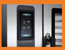
Touchscreen display: The 7-inch TFT HiRes glass touch display delivers brilliant images even at greater distances. Its scroll function and pictograms make operation as easy and intuitive as using a smartphone.
